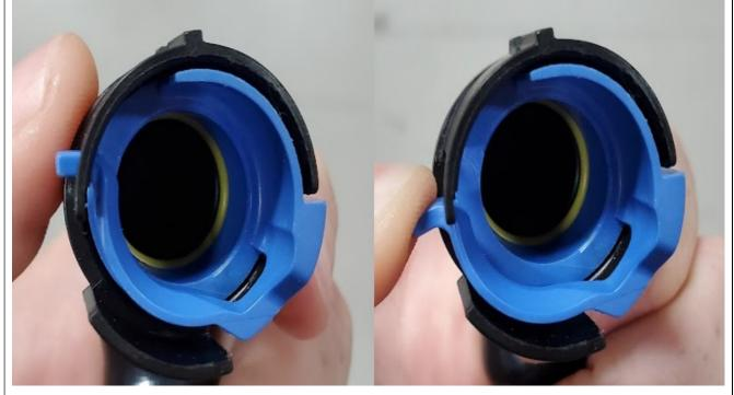
Connect J&L hose to intake first, be sure tab locks into place. Connect J&L male fitting to hose you disconnected from the intake manifold.
