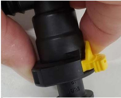
Tab Unlocked, Button pressed to release
